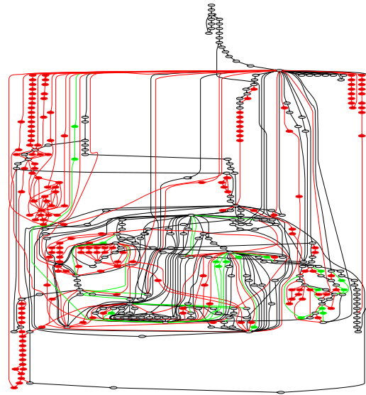
Figure 2: Function-call graph of tiffcp. This figure shows the nodes and edges removed (highlighted in red) or added (highlighted in green) by IgorFuzz.
