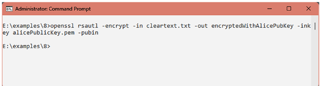
Figure 8-5. Encrypting the clear message and obtaining the encrypted message (a) clear text (b) encrypted text (c) the process of encryption
