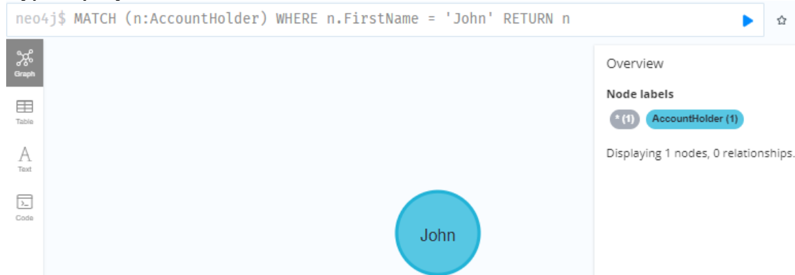
Figure B1: This image shows the result of a standard benign Cypher query. The following images show how each subclass of Cypher injection modifies this query to inject untrusted code in place of the expected FirstName value.
