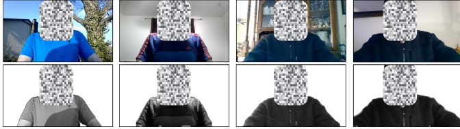
Fig. 17: Example output of the background removal process, using DeepLabv3 and Microsoft COCO, successfully applied in different indoor and outdoor settings. Top four images are the original frames, and bottom four images are corresponding frames after background removal.
