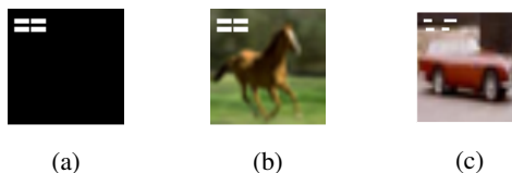
Figure 2: Trigger Examples, (a) is the ground truth trigger, (b) is malicious client poisoned data, (c) is after benign client trigger inversion, augmented data
