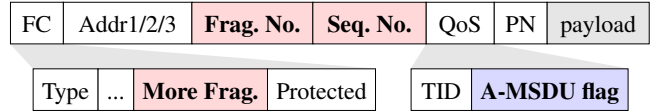
Figure 1: Layout of an encrypted 802.11 frame. Our aggregation attack abuses the field in blue, and our fragmentation attacks the fields in red. Only the payload field is encrypted.
