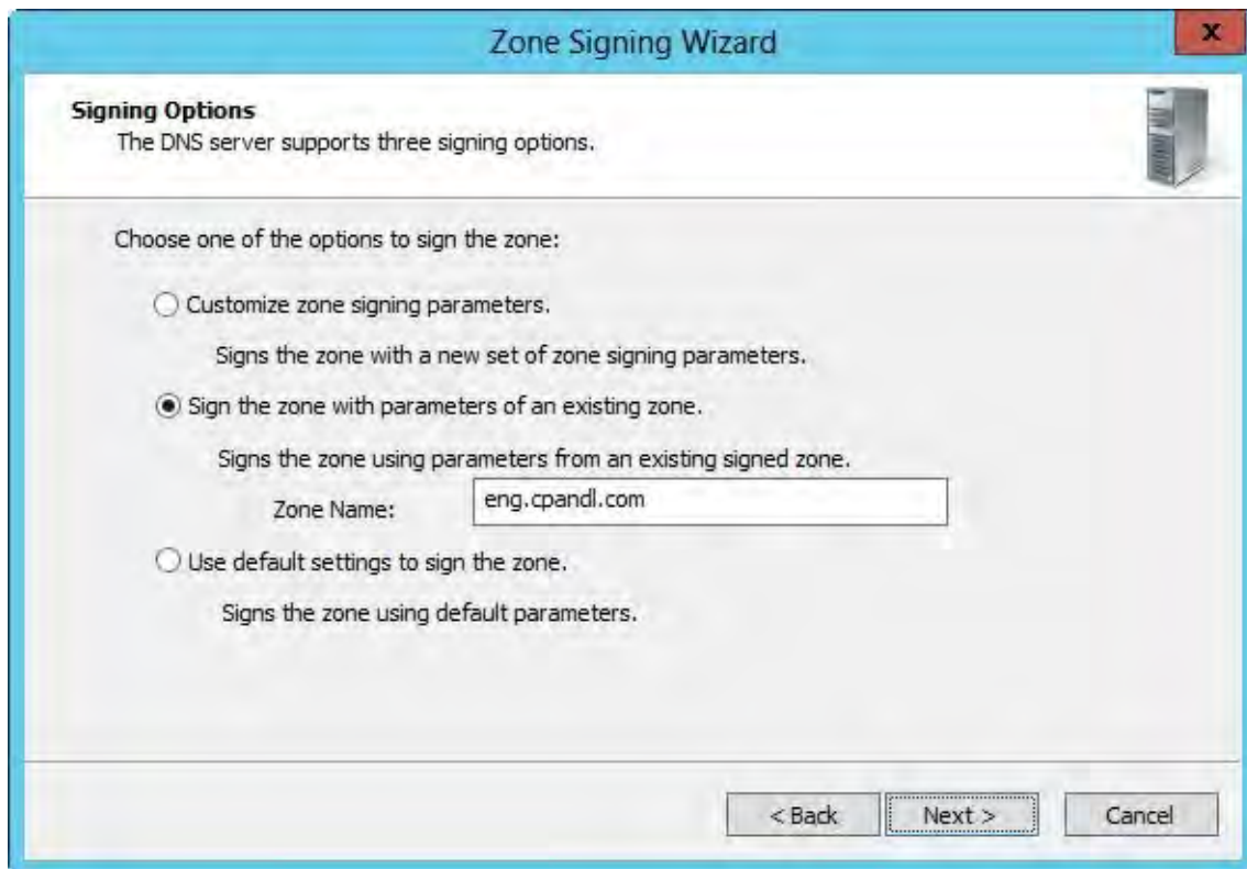
Figure 7-20 Using the settings of another signed zone to quickly set up a new zone.
