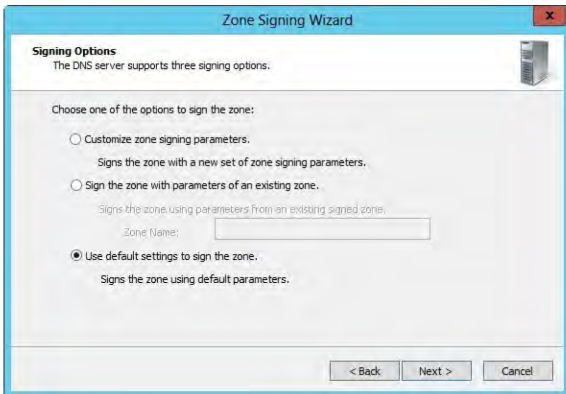
Figure 7-19 Using the default signing options to configure signing automatically.
