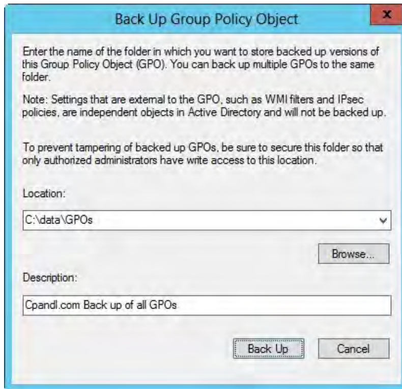
Figure 17-27 Set the backup location and description.
