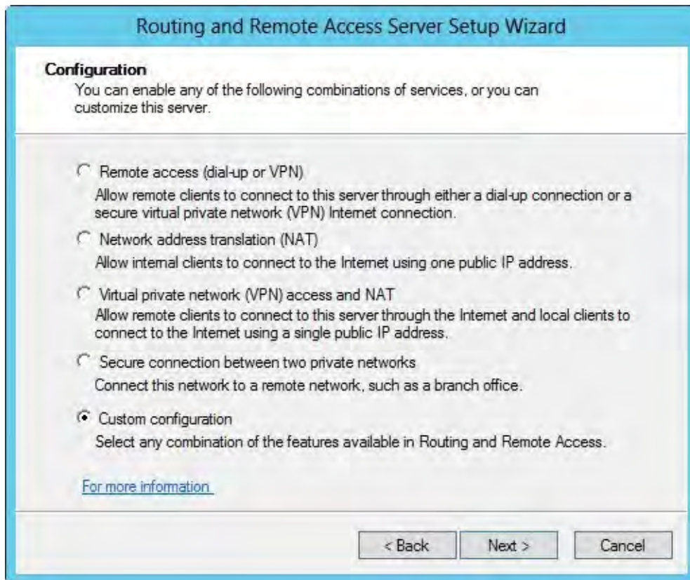
Figure 5-10 Configure and enable Routing And Remote Access.
