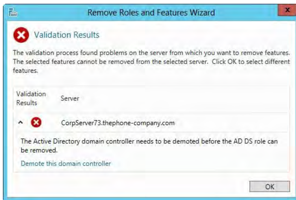
Figure 14-9 Demote the domain controller.
