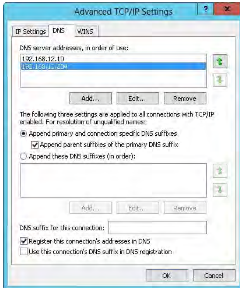
Figure 3-3 Configure advanced DNS settings in the DNS tab of the Advanced TCP/IP Settings dialog box.
