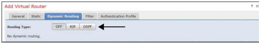
Figure 6-19 Dynamic Routing on a Virtual Router
