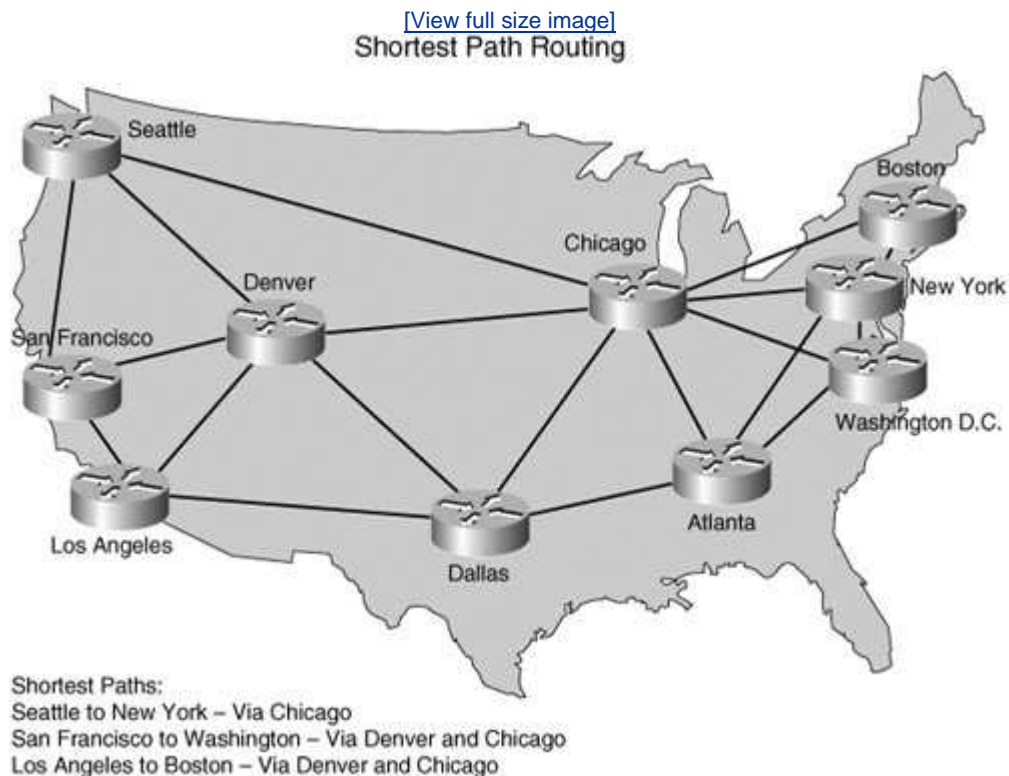
Figure 8-1. Shortest Path Routing
