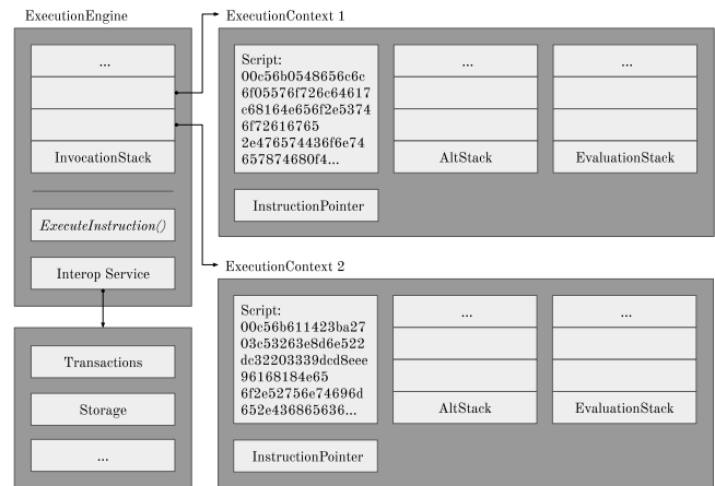
Figure 1: Neo VM architecture: The main component of the Neo VM is the ExecutionEngine . It executes each smart contract in independent ExecutionContexts , ensuring strict separation between smart contracts. Each contract can work on two separate stacks, the AltStack and ExecutionStack . Through the Interop Service , contracts can access external data and state.
