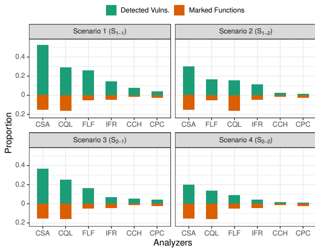
Figure 6: Proportion of detected vulnerabilities and flagged functions (mirrored y-axis scale) by the different static C analyzers in all benchmark programs.
