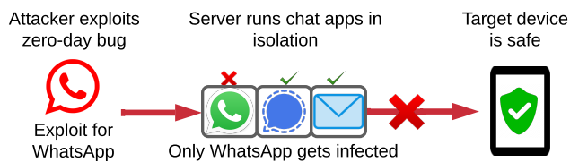
Figure 2: Our attempt at building a Zero-Click Secure Architecture: The user accesses remote isolated chat applications via screen sharing, which confines zero-click exploit to the targeted application only, and safeguards other applications on the server as well as the target device.
