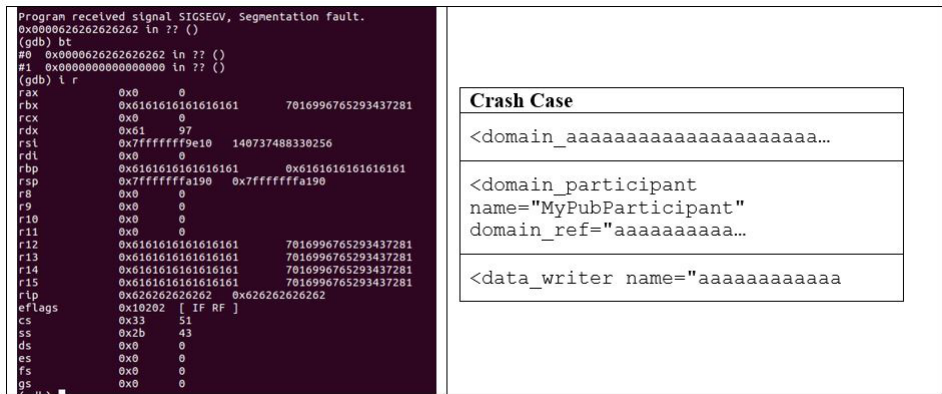
Figure 30. Register state and sample crash cases in RTI Connex DDS Connector (Python bindings) found with RADAMSA from the original XML configuration file.
