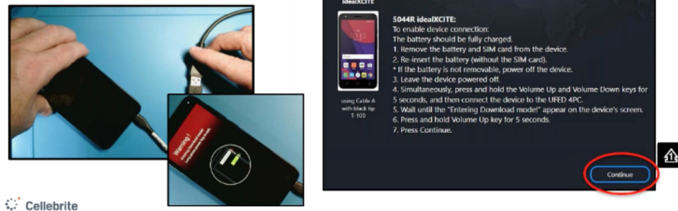
Figure 4.19: Cellebrite EDL Instructions for an Encrypted Alcatel Android Device
