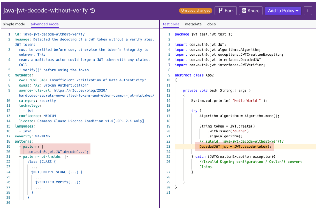
Figure 8.14 – Failure to validate the JWT signature
