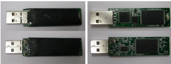
Fig. 12. IronKey S200 before and after epoxy removal
