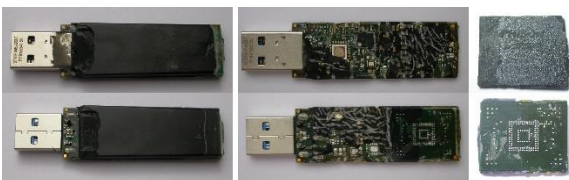
Fig. 22. IronKey S1000 before and after epoxy removal
