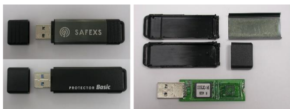
Fig. 59. SafeXS Protector before and after opening its plastic case
