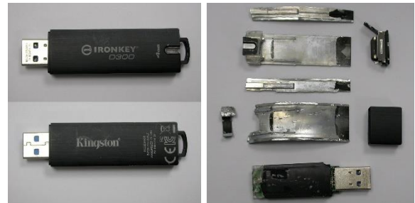
Fig. 23. IronKey D300 before and after opening its metal case
