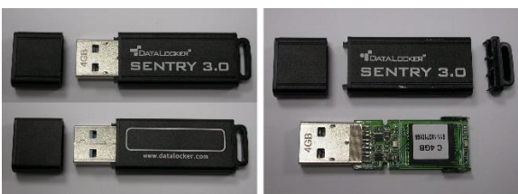
Fig. 54. Sentry 3.0 before and after opening its metal case
