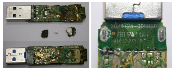
Fig. 24. IronKey D300 after epoxy removal
