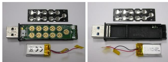
Fig. 39. DataTraveler DT2000 after disassembling the enclosure
