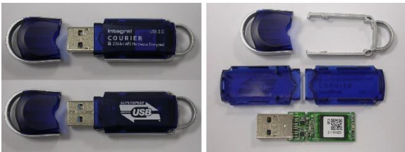
Fig. 52. Integral Courier before and after opening its plastic case
