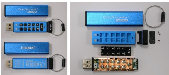
Fig. 38. DataTraveler DT2000 before and after opening its metal case
