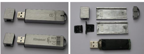
Fig. 21. IronKey S1000 before and after opening its metal case
