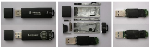
Fig. 26. IronKey D300S before and after opening its metal case
