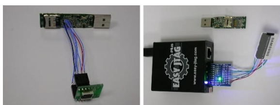
Fig. 61. Testing Serial Flash and microSD card from IronKey F150
