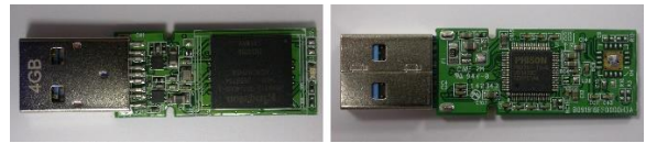
Fig. 55. PCB image of Sentry 3.0
