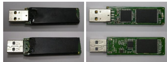
Fig. 17. IronKey D250 before and after epoxy removal
