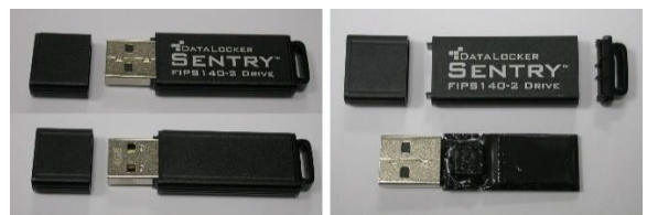
Fig. 56. Sentry before and after opening its metal case
