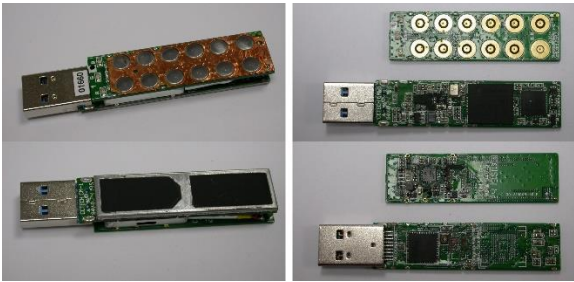
Fig. 44. Datashur Pro2 before and after epoxy removal
