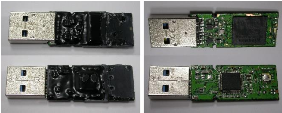
Fig. 51. Integral Crypto before and after epoxy removal
