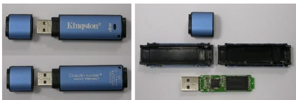
Fig. 36. DataTraveler Vault Privacy before and after opening its plastic case
