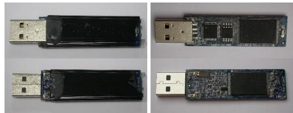
Fig. 9. IronKey D2 Ver.2 before and after epoxy removal
