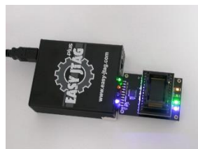
Fig. 62. Testing NAND Flash from IronKey D80
