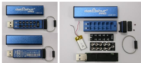
Fig. 41. Datashur Pro before and after opening its metal case
