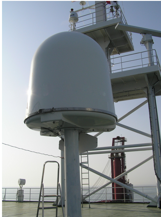
Figure 5.1: A typical marine VSAT system [156].
