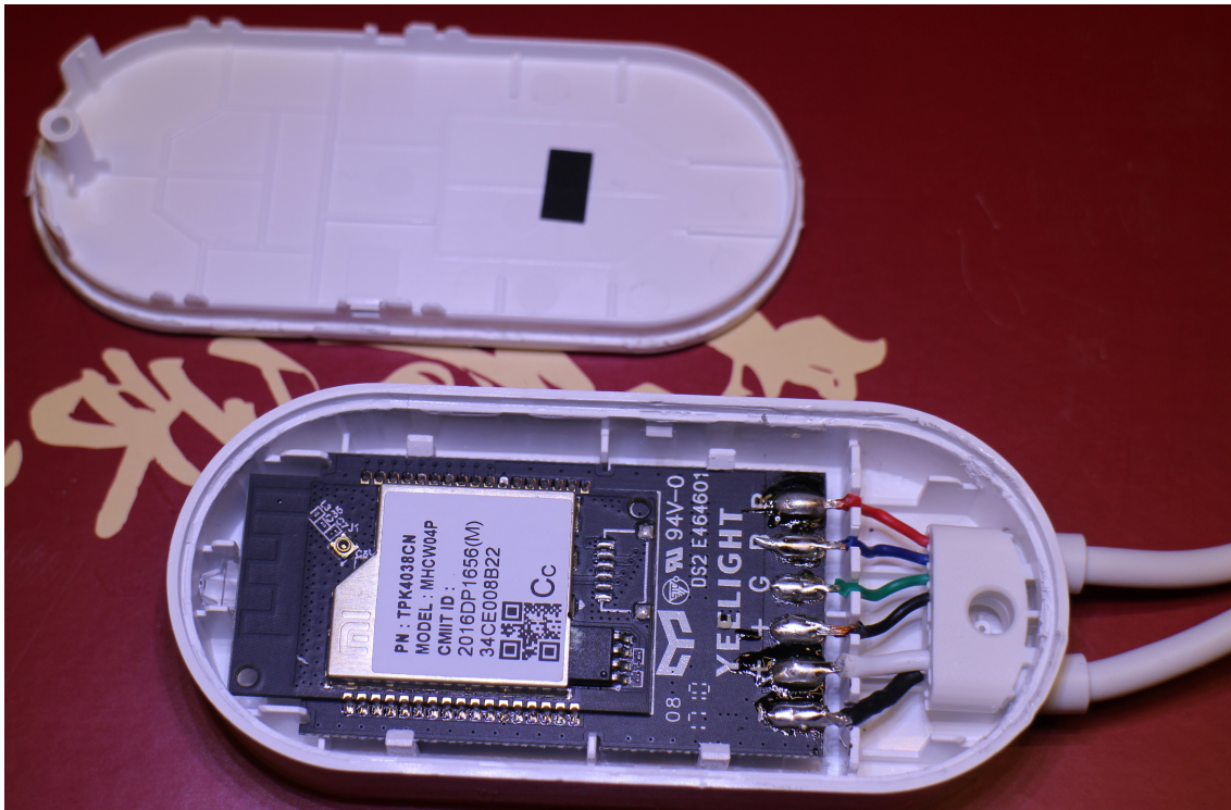
Figure 21: Front side of the PCB in disassembled Yeelight LED Strip
