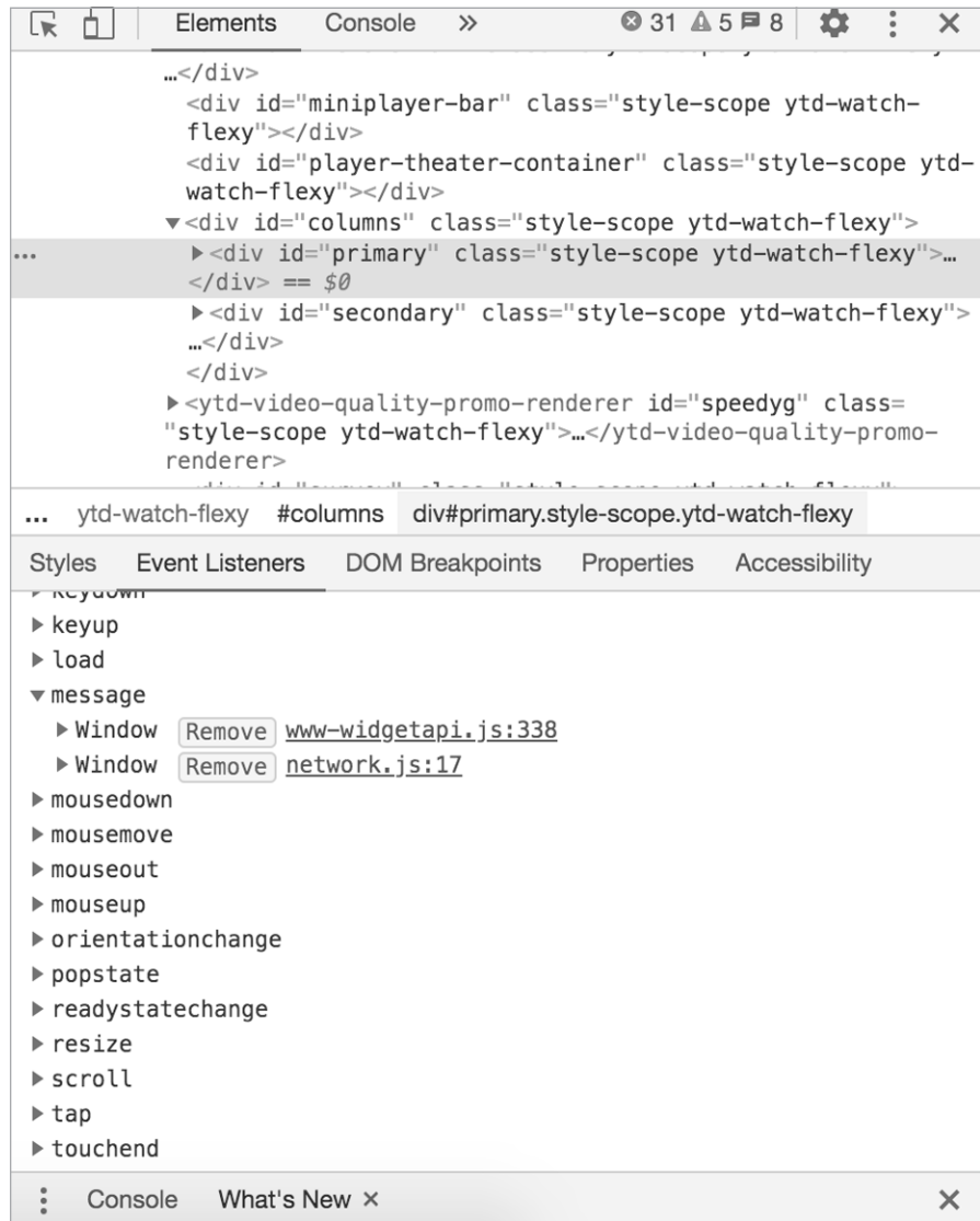
Figure 19-1: Finding the event listeners of a page in the Chrome browser
