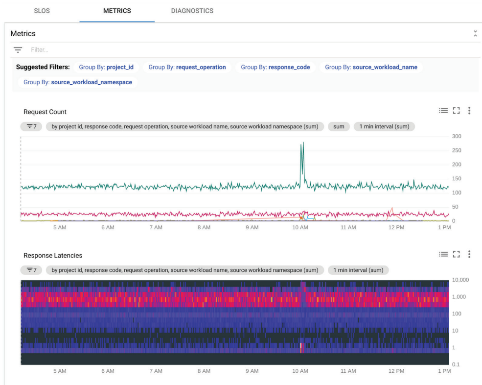
FIGURE 8.1 Service dashboard showing request count and latency time series data
