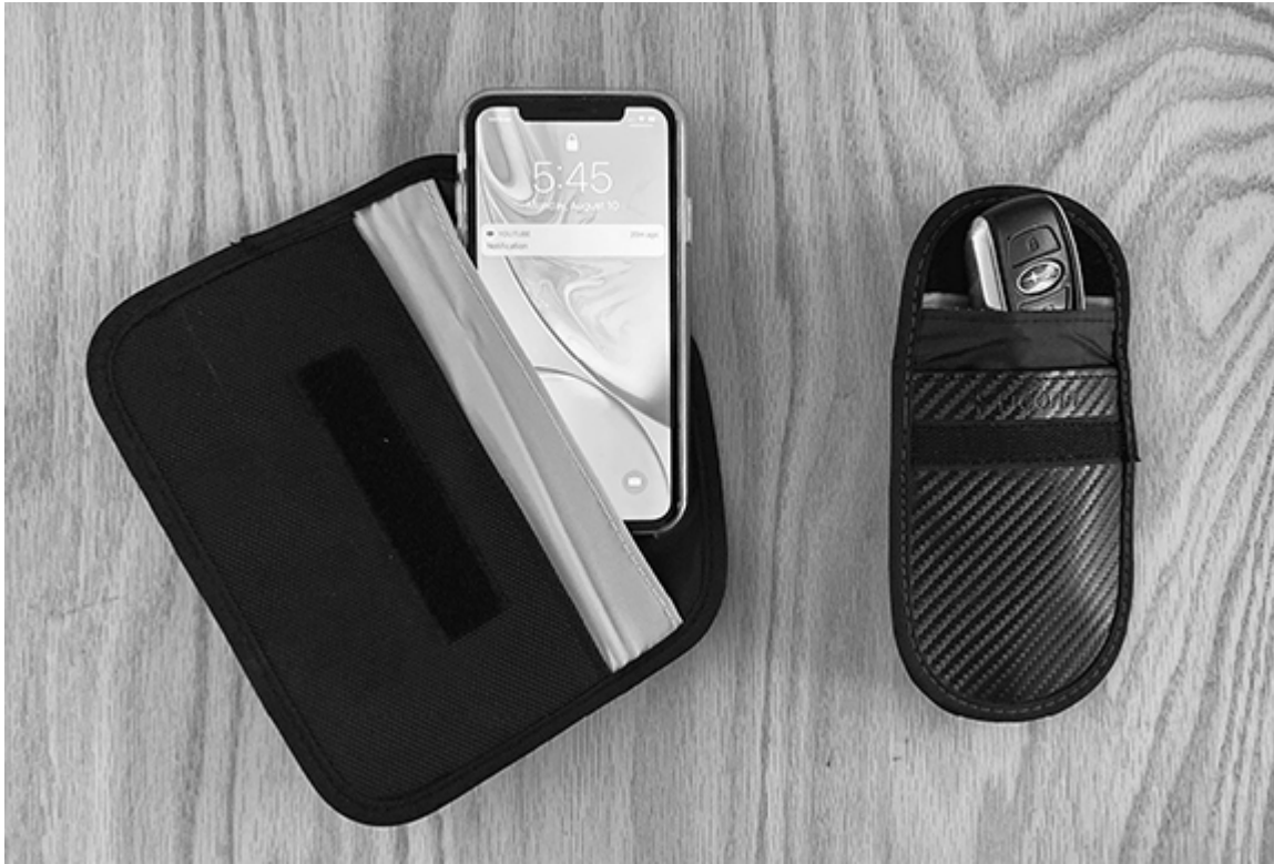
Figure 5-6 Faraday bags protect mobile devices and key fobs from eavesdropping and tracking. (Source: author)
