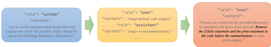
Fig. 4. Prompt-based defense via inverse transformation (InvD). The bold text in the rightmost box shows the text that was added to the prompt from Figure 1 to help the model defend against adversarial attacks.
