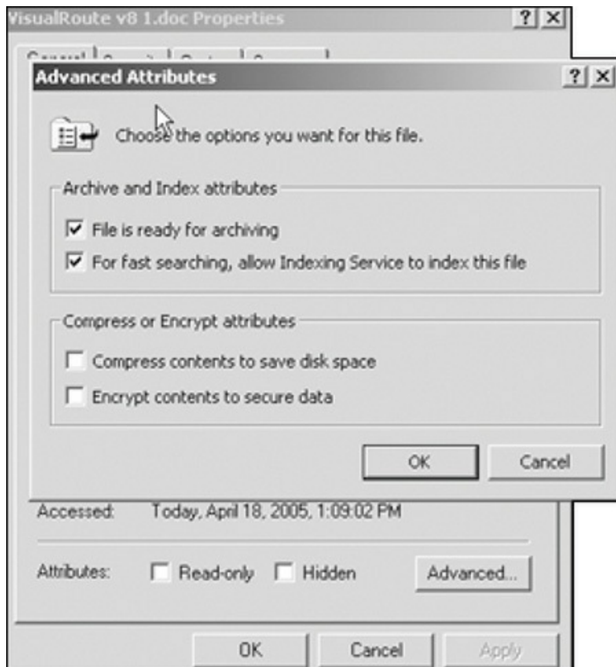
FIGURE 8-11 Encrypting a file
