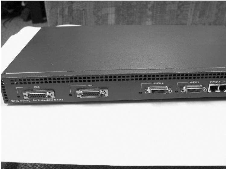
FIGURE 3.13 A router with two LAN ports and two WAN ports.
