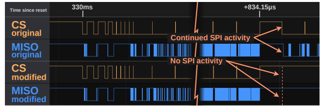
Figure 2: SPI bus traces during the initial boot. CS and MISO lines only. The upper part depicts SPI bus activity for the original flash image (“CS original” and “MISO original”). The lower part shows the corresponding SPI signals for a flash image with a manipulated ARK.
