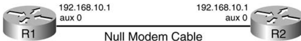
Figure 3-6. Routers Back-to-Back Through the AUX Ports
