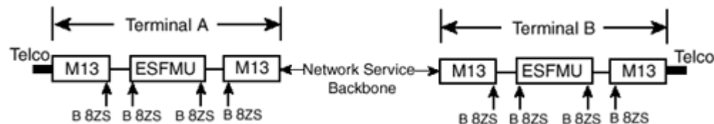
Figure 13-13. End-to-End B8ZS Encoding
