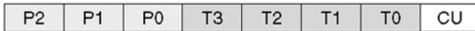
Figure G-1 Internet Protocol (IP) Precedence Bits Type of Service (ToS) Byte
