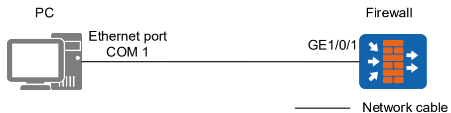
Figure 3-1 Topology for basic firewall configurations
