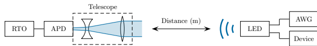
Figure 9: Experimental setup for exfiltrating data in two different setting: First, driven by an arbitrary waveform generator (AWG) and second, operated by the targeted device. Signals are captured with an avalanche photodetector (APD) and processed with a real-time oscilloscope (RTO).
