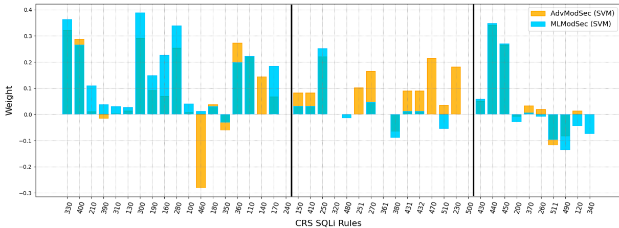
Figure 7: Weight values learned by MLModSec SVM (cyan) and AdvModSec SVM (yellow). The additional color, i.e., turquoise, is given by the overlapping of the yellow bars with the cyan ones. For brevity and clarity’s sake we only report the last three digits of the rule IDs on the x-axis since, for all the rules, the first three digits are equal to 942.
