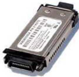
Figure 6. Gigabit Interface Converter (GBIC)
