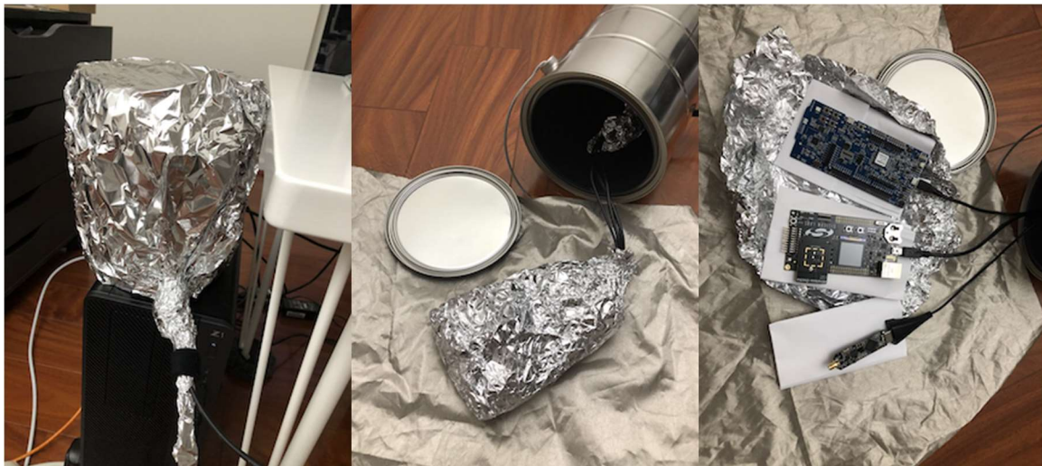
Figure 7. Baked-potato style Faraday cage
