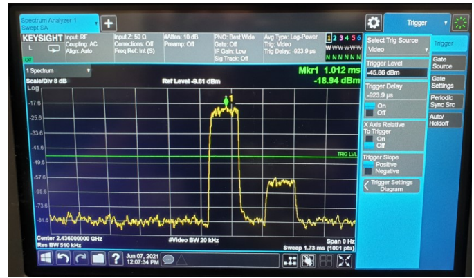
Fig. 1. Alice (left) and Bob’s (right) packets observed on spectrum analyzer. Time between Alice’s packet to Bob’s packet is approximately 150\mu\text{s} . The round-trip-time is approximately 480\mu\text{s} .
