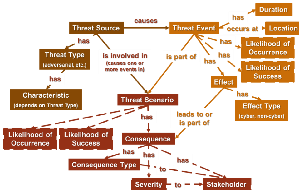
Figure 16. Key Constructs in Cyber Threat Modeling (Details for Adversarial Threats Not Shown)
