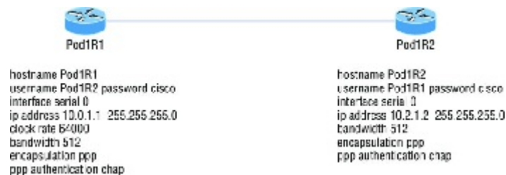
FIGURE 21.17 Mismatched IP addresses
