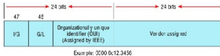
FIGURE 2.7 Ethernet addressing using MAC addresses
