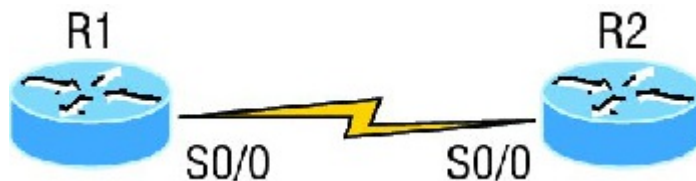
FIGURE 6.6 By looking at R1, the show controllers command reveals that R1 and R2 can't communicate.
