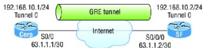
FIGURE 21.24 Example of GRE configuration
