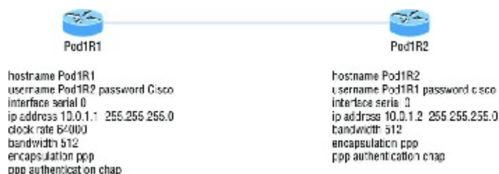
FIGURE 21.15 Failed PPP authentication
