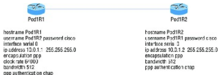
FIGURE 21.14 PPP authentication example
