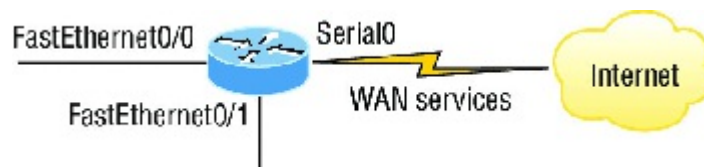
FIGURE 1.15 A router in an internetwork. Each router LAN interface is a broadcast domain. Routers break up broadcast domains by default and provide WAN services.
