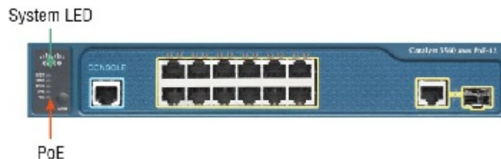
FIGURE 10.9 A Cisco Catalyst switch
