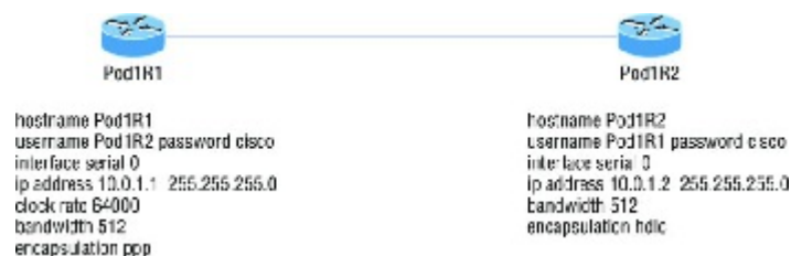
FIGURE 21.16 Mismatched WAN encapsulations
