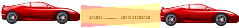
Figure 11.3. Communication by light between two vehicles. For a color version of this figure, see www.iste.co.uk/haddadou/edge.zip
