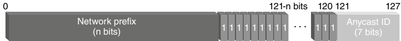
Figure 17.11 Reserved subnet anycast address format when EUI-64 is not required. Source: Based on Mrugalski et al. 2018 [20].
