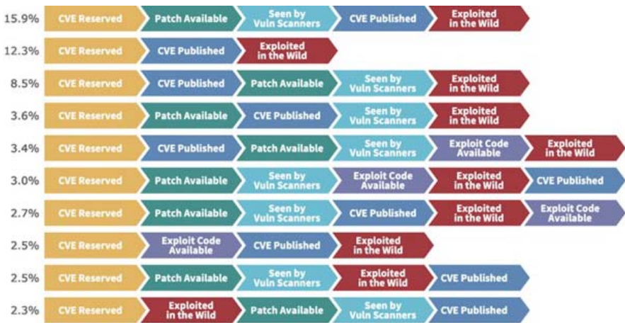
Figure 5.14 Top 10 sequences of key milestones in the vulnerability lifecycle. (© 2021 Kenna Security/Cyentia Institute. Reprinted with permission [9].)
