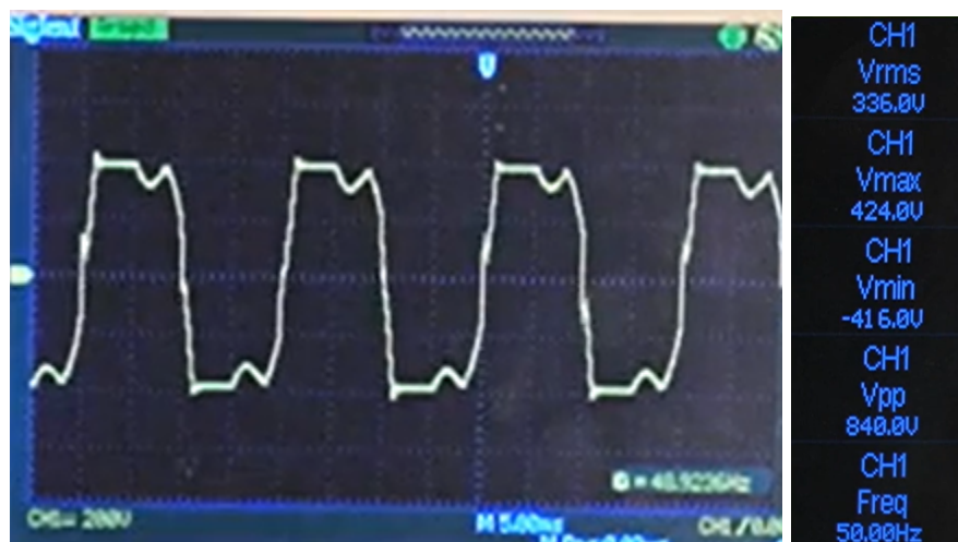
UPS output of square wave taken from oscilloscope. V_{rms} reached 336 Volts.
