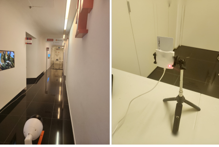
Fig. 7. Experimental setup. As seen on the left, the video camera was directed at the smart card reader (indicated by the red arrow) from 16 meters away. On the right is an image of the smart card reader’s power LED.
