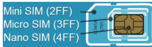
Figure 2: SIM Card Size Formats [Orm09]
