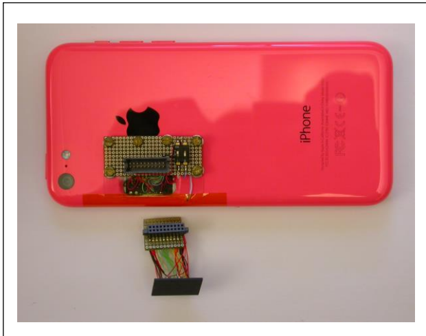
Figure 10. iPhone 5c with NAND on connector
