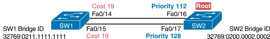
Figure 8-7 The Need for Additional Root Port Tiebreakers
