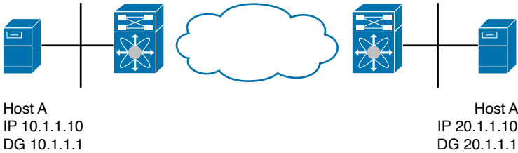
Figure 20-7 Two Hosts in Different Subnets
