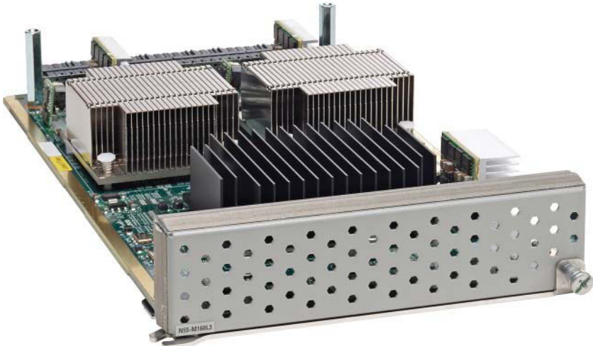
Figure 1-46 Cisco Nexus 5596UP Layer 3 Daughter Card Upgrade Procedure
