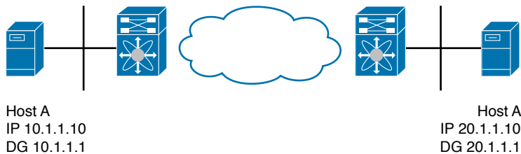
Figure 20-2 Communications Between Two Hosts in Different Subnets
