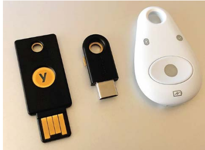
Figure 3.19 – Hardware token and key fob used with a proximity card
