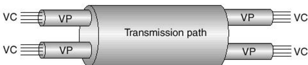
Figure 2-12. ATM Virtual Circuits from a Customer Perspective
