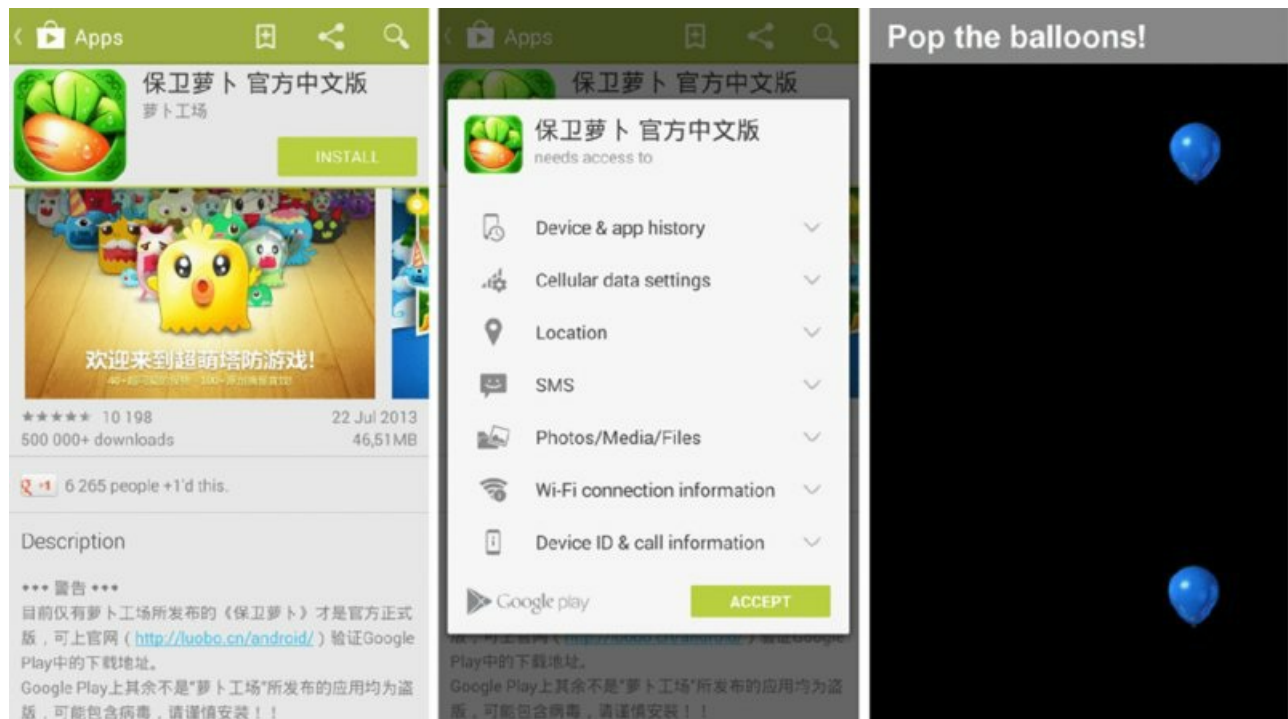
Figure 7.5 An illustration of how a toast could be used to perform unintended actions on underlying activities
