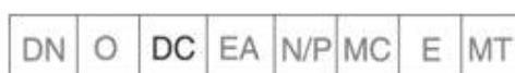
Figure 8.39. The DC bit in the Options field indicates support for DoNotAge LSAs.
