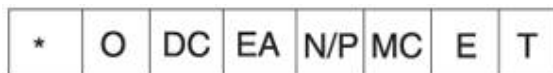
Figure 7.20. The E bit in the Options field of the OSPF Hello messages is set to indicate support of external routing capability (a nonstub area) and is cleared to indicate nonsupport of external routing capability (a stub area).
