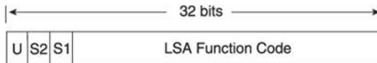
Figure 12.8. Details of the Link State Type field in the OSPFv3 LSA header.
