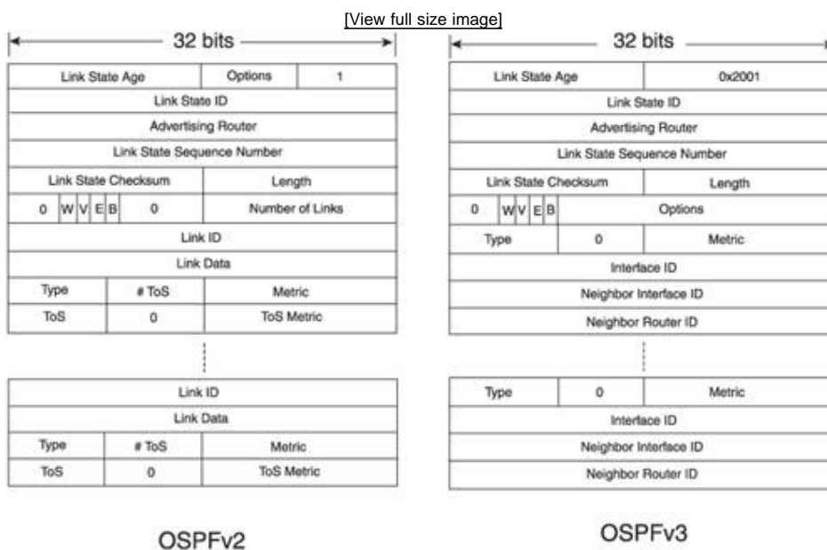
Figure 12.12. Comparison of the OSPFv2 and OSPFv3 Router LSAs.
