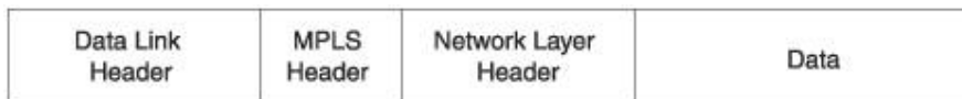
Figure 11.4. The MPLS header is added to the front of the network layer packet to be encapsulated, and is then encapsulated by the data link header.
