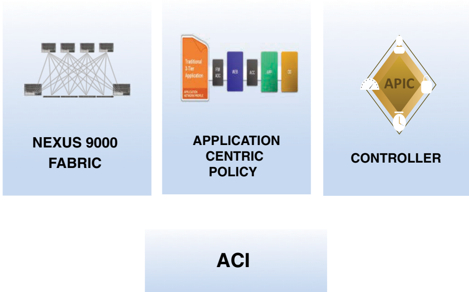
Figure 3-4 ACI Building blocks
