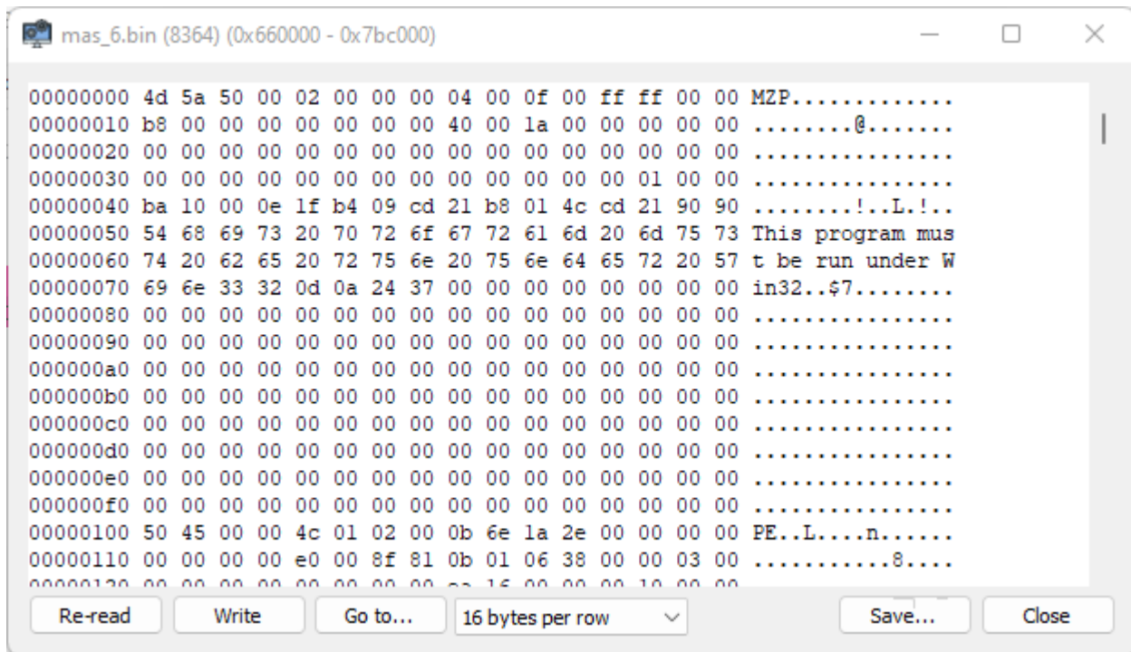
[Figure 31] System Informer (Process Hacker): visualizing the PE file in the region
